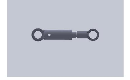
To assemble the side tubes, thread the M2 3.5mm Ball cup onto the damper piston. We suggest 15,000-20,000 grease to start with these new and improved dampers.
