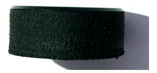
It is possible that a burr of the injection point remains on the inside of the sidewall. This can compromise the proper functioning of the part since it will not be continuously supported on the sidewall of the tire.
