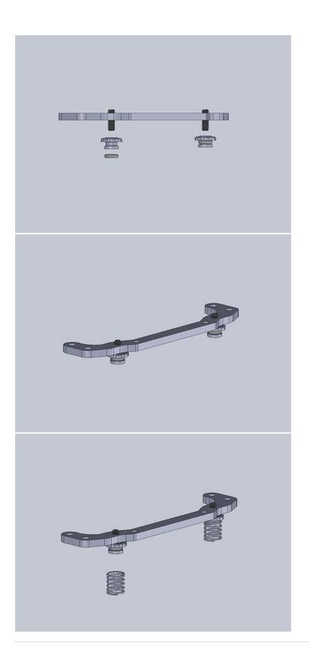
Now we install the Spring Perches. It is important that in this step, you use some Thread Locker on the set screws before installing the spring perch. Failure to do so will not allow the setting of tweak to hold.
