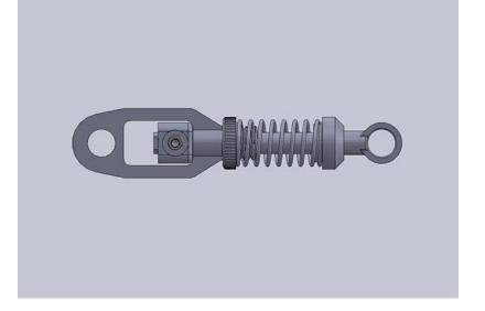
Assemble the Center Shock in the order illustrated on the left. Apply some 30,000 lube on the shock shaft to start.
