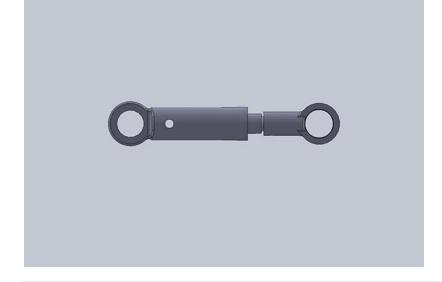
Pop the center shock onto the Pivot Balls with the spring side towards the back. Place the car on a flat surface and then adjust the droop collar so that there is a 0.5mm gap between the droop adjustment collar and the shock body. This will give you 0.5mm of droop.
